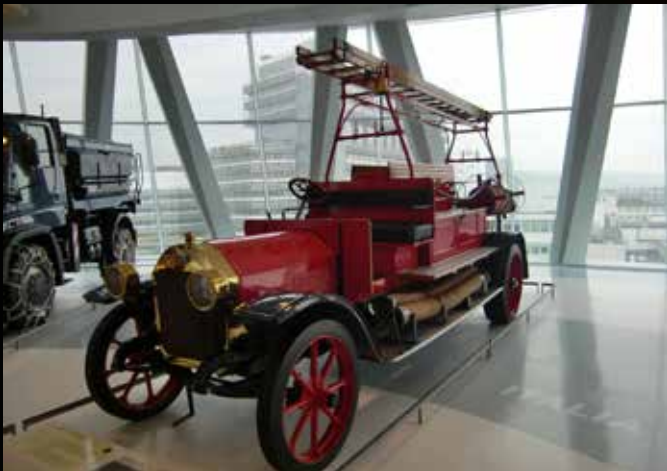
Benz Motorspritze, 1912, 4 Zylinder, 8588 cm 3 , 58 PS, 40 km/h
