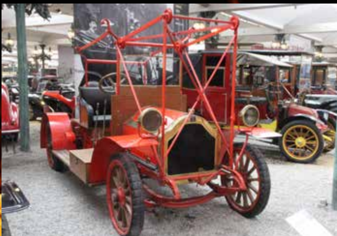
Benz Motorspritze, 1912, 4 Zylinder, 8588 cm 3 , 58 PS, 40 km/h
