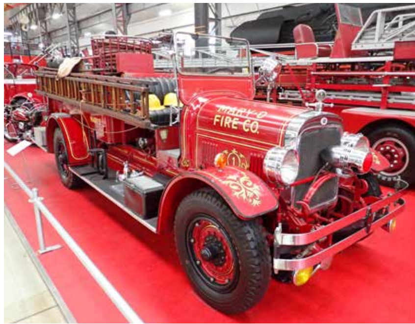
Seagraves Pumper, Baujahr 1961, 6 Zylinder, 6.000 ccm, 90 PS
