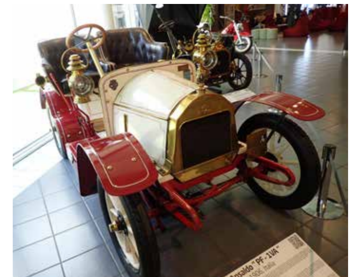
Ansaldo PF-1VA, Bj. 1906, 1 Zylinder, 850 ccm, 45 km/h
